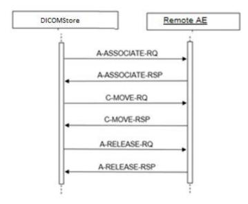
Figure 8: Data Flow Diagram - MOVE as SCU
