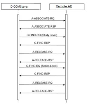
Figure 7: Data Flow Diagram - FIND as SCU
